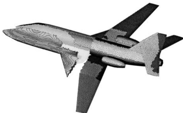
FIGURE 5. An extract of a solution of Maxwell equations on a perfectly conductive airplane  $\Gamma$  and the partitioning into 8 processes.
