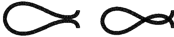
FIGURE 8. Comparison of the equilibrium states obtained with \gamma = 0.1 when self-contacts are taken into account (left) or not (right).
