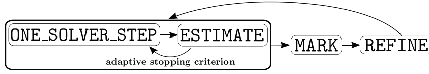
Scheme 2. Paradigm of an adaptive loop employing an inexact algebraic solver.
