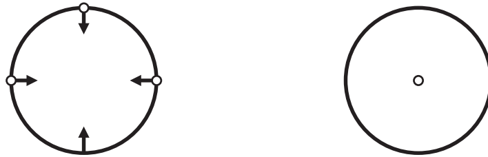
FIGURE 1. Left: contractive forces are defined on the cell boundary in the point force approach. Right: point stress approach employs an isotropic stress point source in the cell center.
