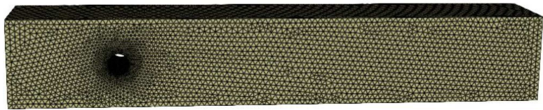
FIGURE 5. Test 3: surface view of the computational mesh.
