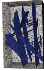
FIGURE 7. Large DFM model meshed with 495 233 tetrahedra and 66 908 fracture faces.
